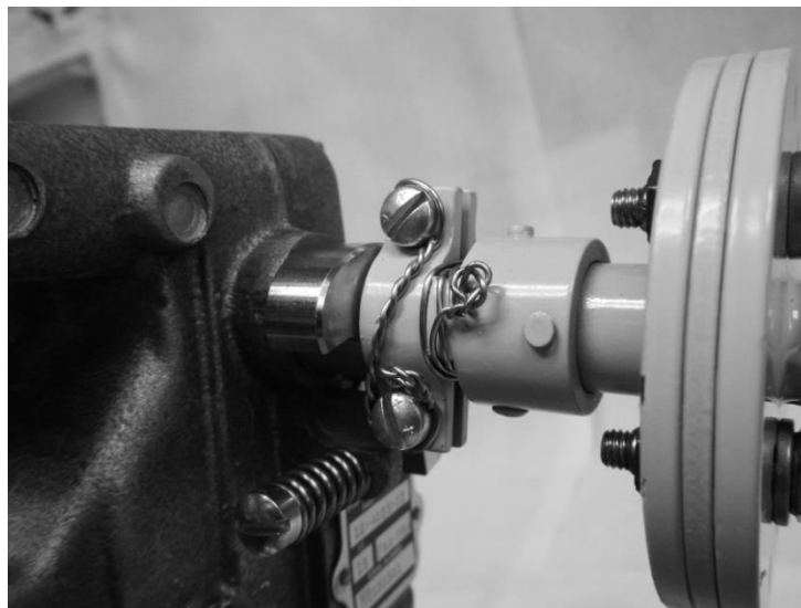
Figure 5-6e: Securing Throttle Linkage Adapter to Carburetor Stop Arm with Safety Wire
